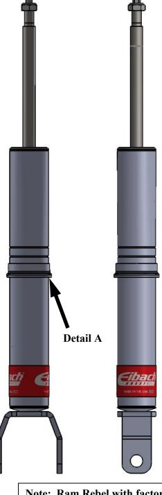
Note: Ram Rebel with factory Bilstein shocks will not use the Spring Perch Adapter
